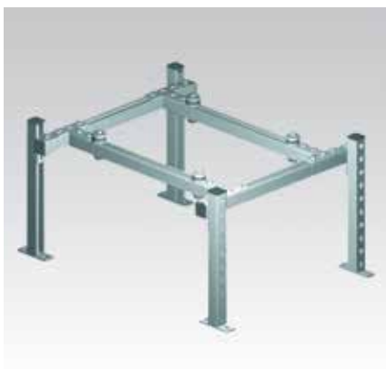
Frame construction consisting of MPC-Support channels, MPC-Wall hanger brackets, mounting angles, short and connection plates
