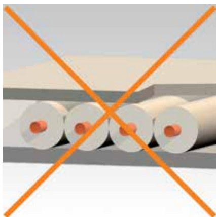
Insulation tube: large floor height required
